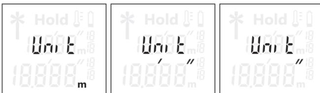
Hold down the on/off button (1). When the required unit of measure is displayed, release the on/off button (1). After releasing, the measuring tool switches itself on with the selected setting.
